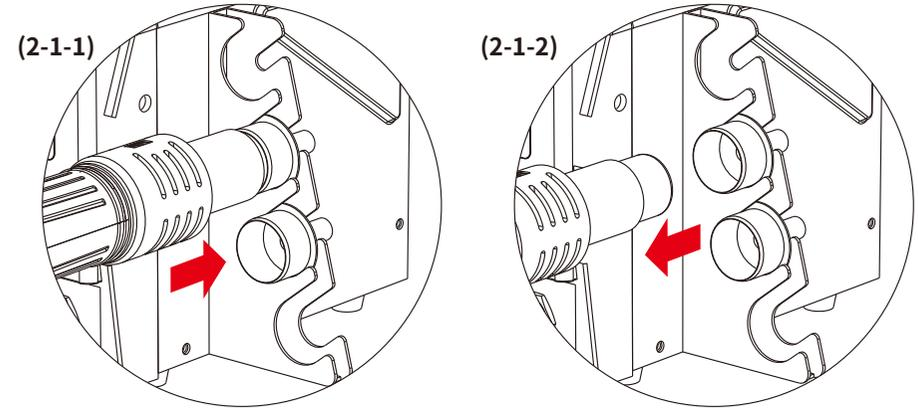
Illustrations of Incorrect Removal of the Hot Air Gun Nozzle.
